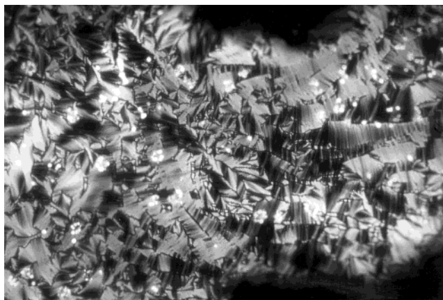
Figure 1. Fan-shaped texture of the spiro compound 3f as seen between crossed polarizers at 100°C upon cooling ( \times 250 )
