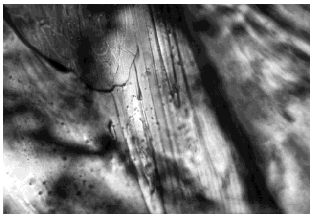
Figure 2. Spread sample of the tetramer 7f as seen between crossed polarizers at 22^\circ\text{C} ( \times 250 )
